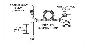
FIGURE 20. GAS PIPING WITH FLEXIBLE CONNECTOR.
